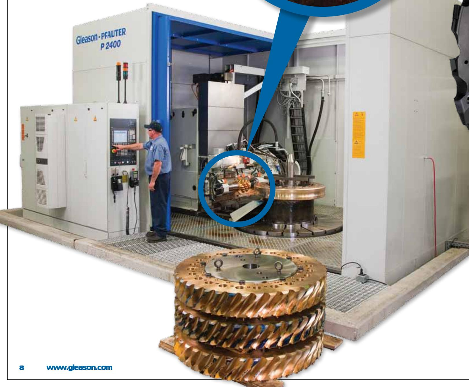
While machine design and construction are important considerations, Mr. Hupp says that the special design of the hob doing the cutting is the most decisive factor. For 100 years, Cleveland Gear has designed, developed and manufactured its own hobs. In fact, hobs are numbered in a sequence that dates back to hob #1 made in 1912. Today, on the new Gleason-Pfauter P 2400, hob #1924 is in use – a hob that was developed by Gleason Cutting Tools Corporation.
